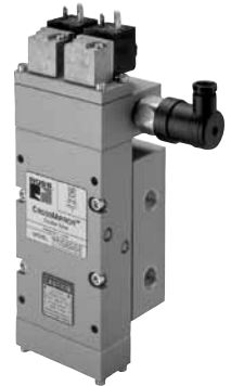
Series 77 CROSSMIRROR® 5/2 double valve for cylinder applications. Sizes 2 and 4 - port sizes 1/2” - 3/4”.
