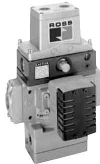
Series 35 - SERPAR® 3/2 double valve with internal monitoring available with L-G, E-P, or D-S monitoring options. Sizes 8, 12 and 30 - port sizes 1/2” - 1 1/2”.
